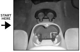
**STEP 1:** Remove the front cup holder to reveal two 18mm bolts. Remove these bolts.
